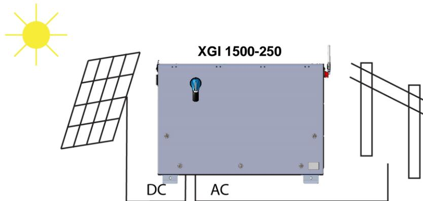
**Figure 2-1 Inverter Usage**
