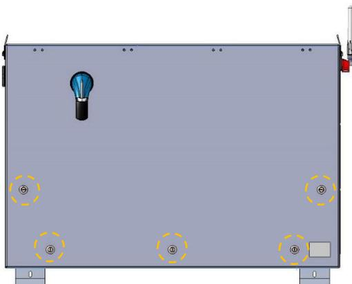
**Figure 3-6 Inverter Cover Latches (Quantity 5)**
