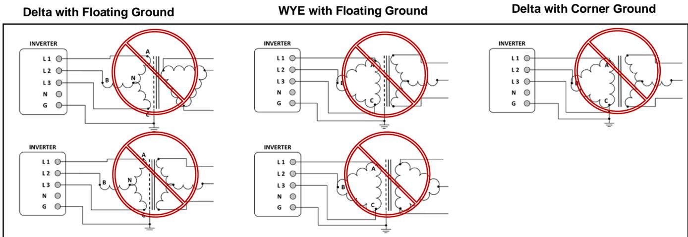
**Figure 3-111 Prohibited Transformer Configurations**
