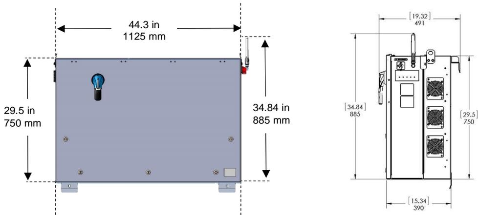
**Figure 3-1 Inverter Dimensions**
