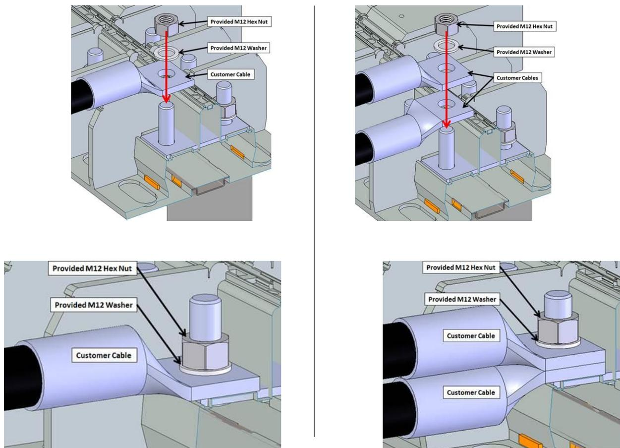
**Figure 3-13 Installation of Single or Parallel Conductor Sets**
