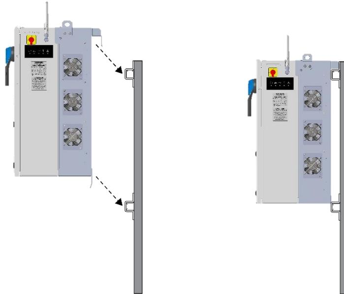
**Figure 3-4 Mounting the Inverter to the Strut Channels**
