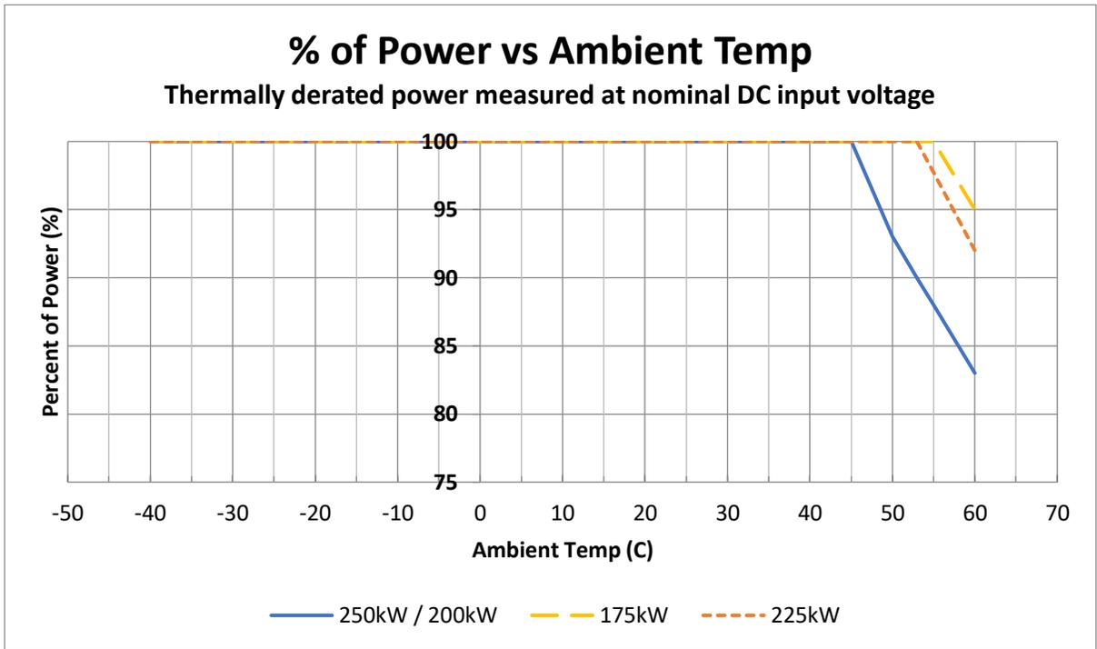
**Figure 10-3 Derating with Temperature**
