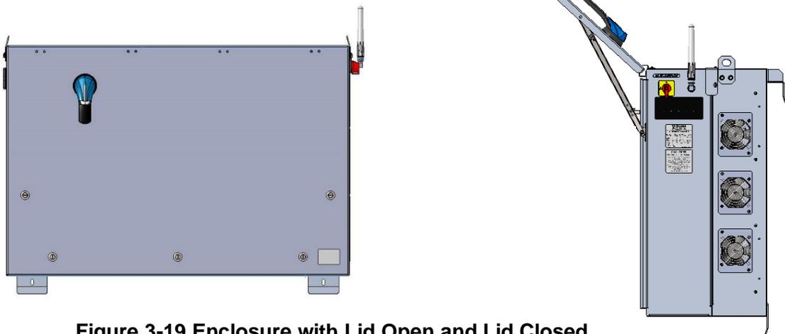
Figure 3-19 Enclosure with Lid Open and Lid Closed
