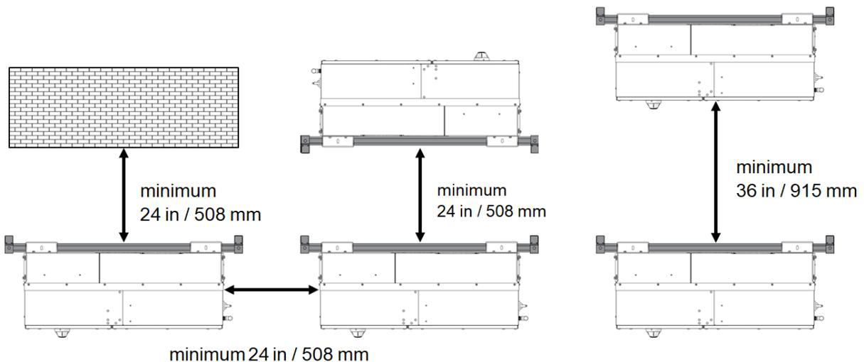
**Figure 3-2 Inverter Minimum Spacing and Mounting – Top View**
