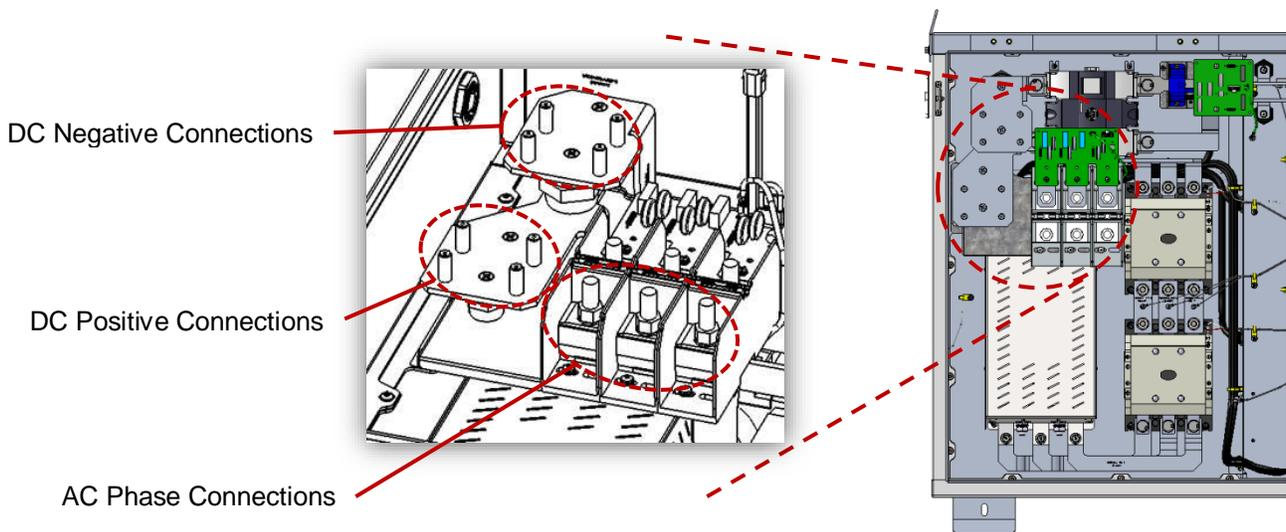
**Figure 3-8 Wiring Box Power Connections**
