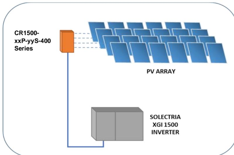
Figure 11-1 Illustration of XGI 1500 Combiner Usage
