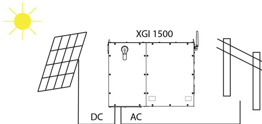
**Figure 2-1 Inverter Usage**
