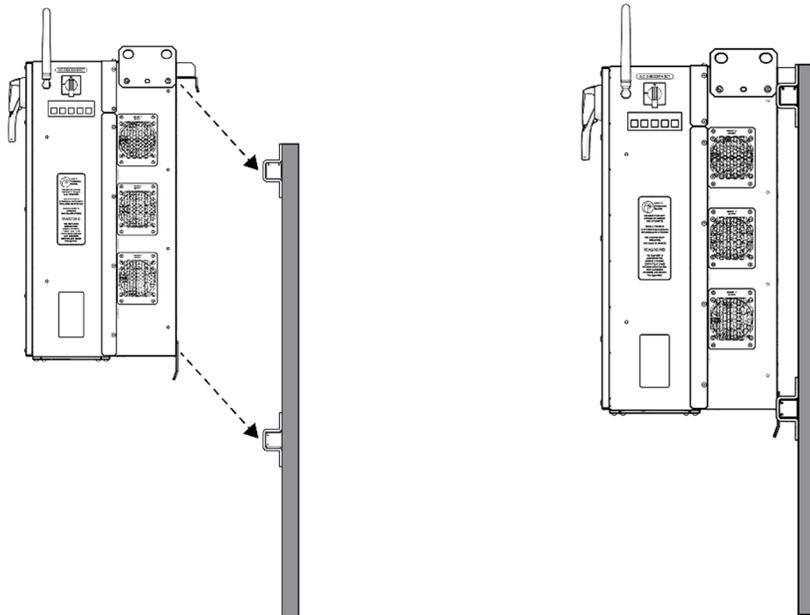
**Figure 3-4 Mounting the Inverter to the Strut Channels**
