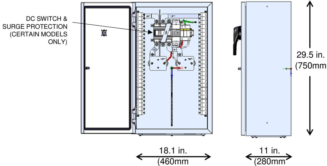
**Figure 11-4 SOLECTRIA XGI 1500 Remote Combiner Box**
