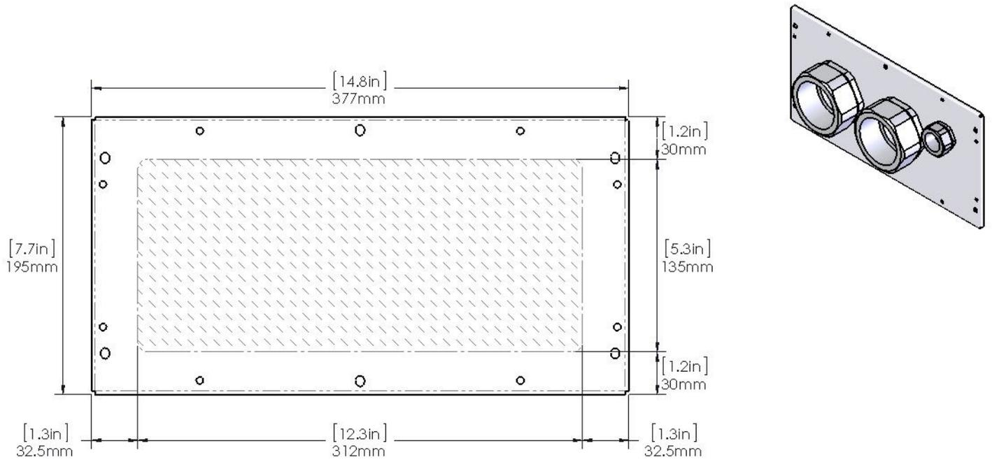
**Figure 3-8 Removable Conduit Panel – Entry Locations**
