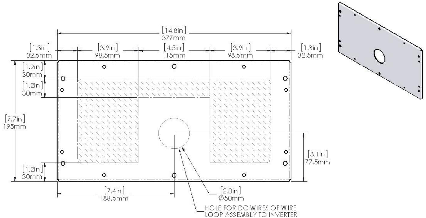
**Figure 3-10 Conduit Hole Location for Attachable Combiners**
