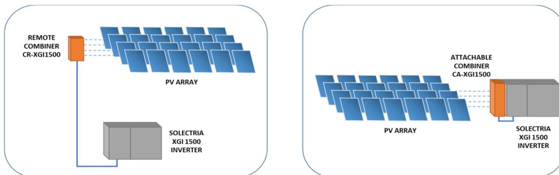
**Figure 11-1 Illustration of XGI 1500 Combiner Usage**
