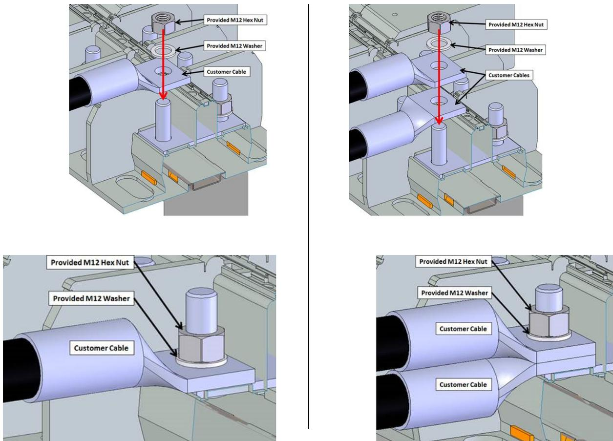
**Figure 3-16 Installation of Single or Parallel Conductor Sets**
