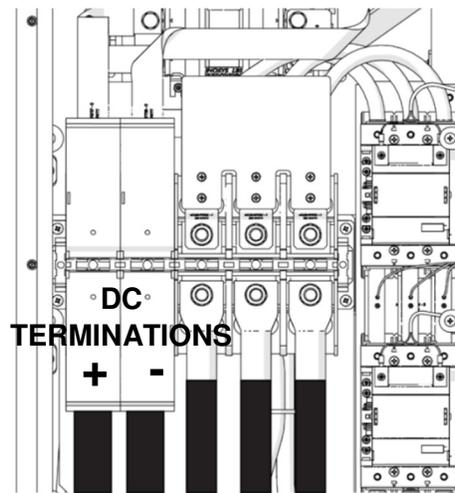
**Figure 3-15 DC Connections from an XGI Remote Combiner**
