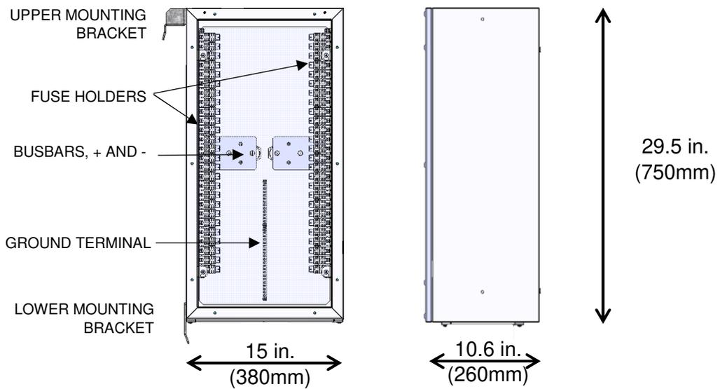
**Figure 11-3 SOLECTRIA XGI 1500 Attached Combiner Box**
