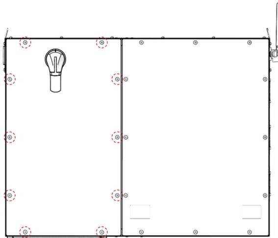
**Figure 3-6 Wiring Box Cover Screws (Quantity 10)**
