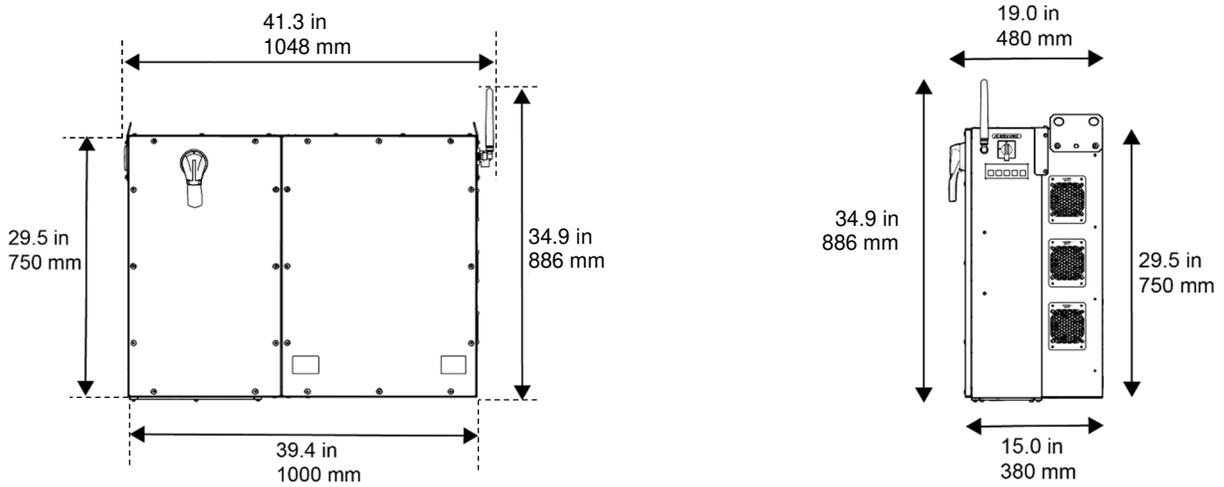
**Figure 3-1 Inverter Dimensions**
