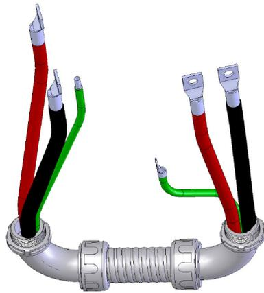
Crimp lugs for terminations on posts in Combiner and XGI wiring compartment.
