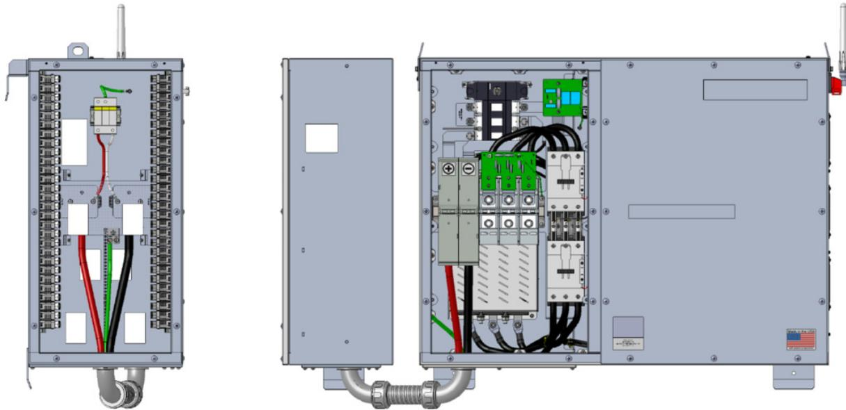
**Figure 3-17 XGI 1500V with Attachable Combiner Box Option**
